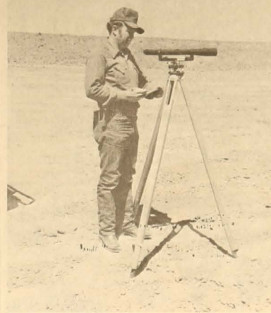
FINAL CHECKOUT —J.K. "Bud" Siebert, Conservation Technician, is shown during a terrace check-out survey. The outlet terraces are designed to hold 2 inches of runoff water.
