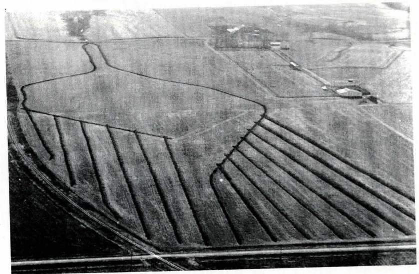
Aerial photo of 980 rod tiling system on J. J. Boatman farm, 5 miles southeast, Montezuma. Over 140 miles of tile were laid in Poweshiek County in 1960.
