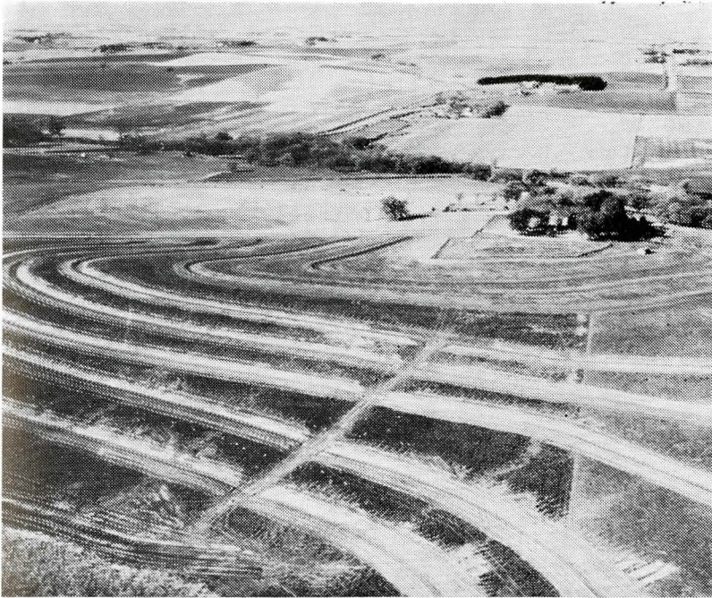
One of the early parallel terrace systems constructed in Cass County was on the Wendell Pellett farm, northwest of Atlantic. Where slopes vary considerably, portions of the terrace system can be made parallel but it is necessary to have corrections to allow for the unevenness of slopes.
