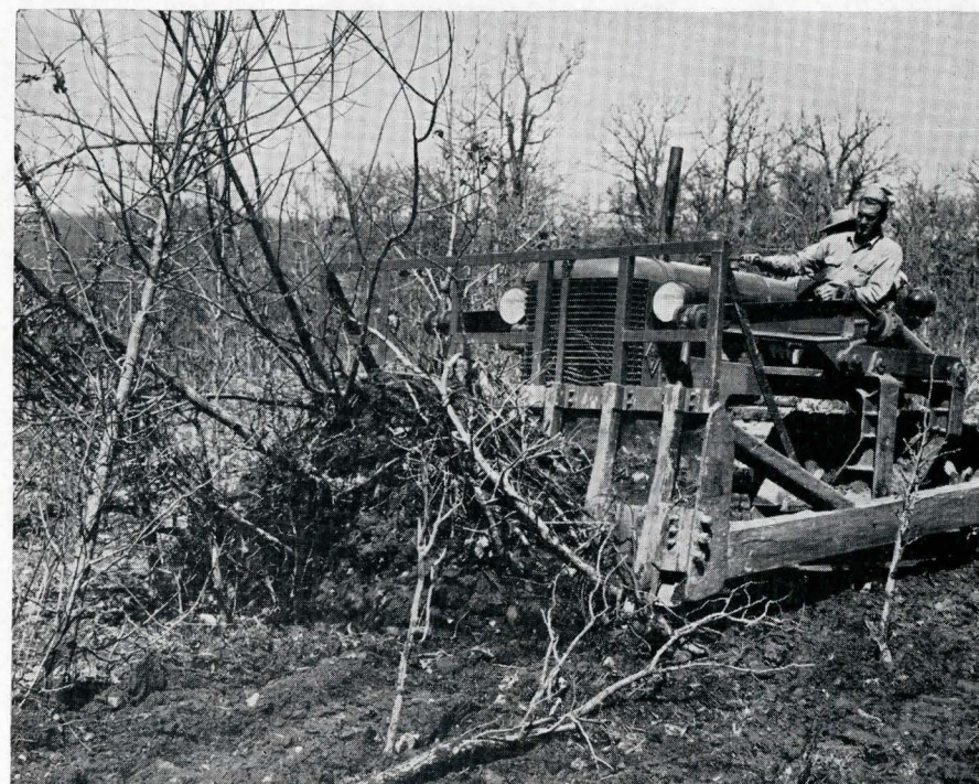
Figure 12. —An Arkansas farmer is clearing brush with a special brush rake attached to a bulldozer. After the brush is removed, he expects to plant a mixture of grasses and legumes.
