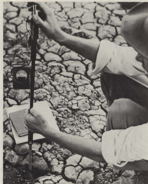
A soil scientist uses a piezometer to find out how far below the surface the ground water lies.
