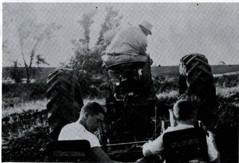
Planting evergreen trees--Lauren Wright farm, Montezuma. Steven Wright & Jimmy Wilcox place trees in slit made by planting machine, while Wright maintains tractor speed at a steady creep.
