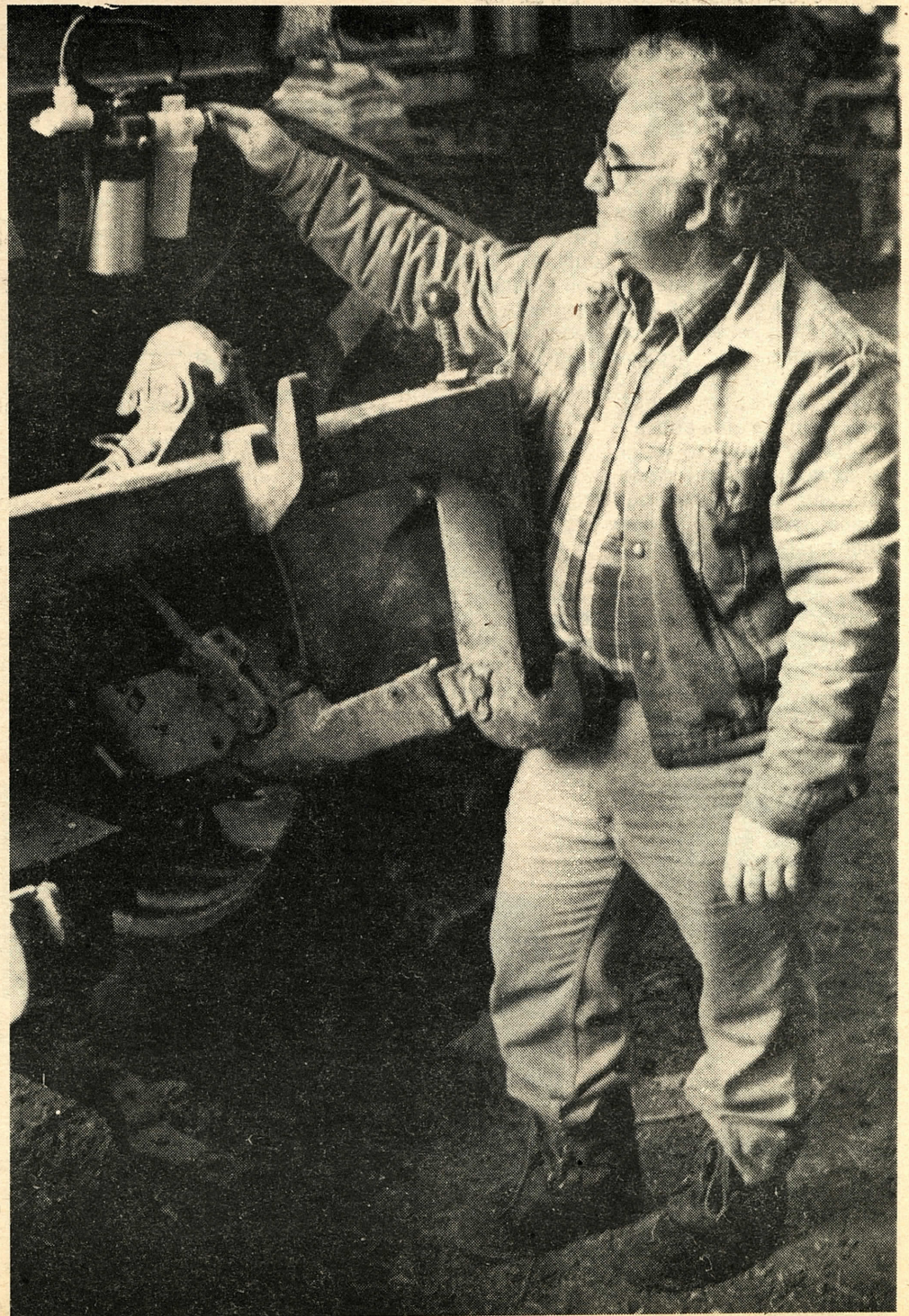
Bob Schott looks over the direct drive fertilizer he uses with his bean drill and electric pump that circulates the liquid corn planter.
