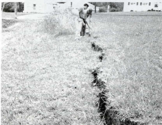
We get all kinds of calls in our new responsibilities with urban land use problems. Harry Bryant takes a look at damage done to a black topped parking lot after an earth slide caused by the long rainy spell. Oren Champ helps Harry check the depth of earth slippage, which later slid several feet farther causing Division Street to be closed for extensive repairs. Soil information can be highly useful to city land users to help avoid such problems before they occur.
