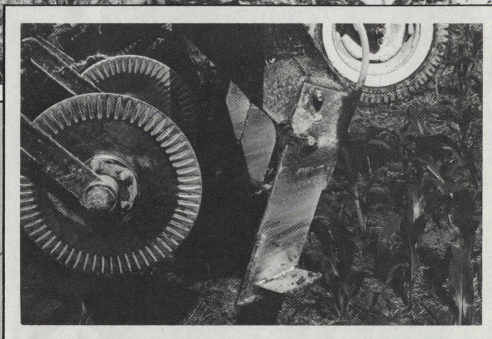
Mike Strohm removes compaction and aerates the soil under growing crops with a tool, above, he designed. The West Union, Ill., farmer uses a toolbar with five 24-inch knives that run 16-inches deep. At right, the coulters cut residue ahead of each knife. Wings 2 inches from the bottom of each knife help lift and break subsoil.
