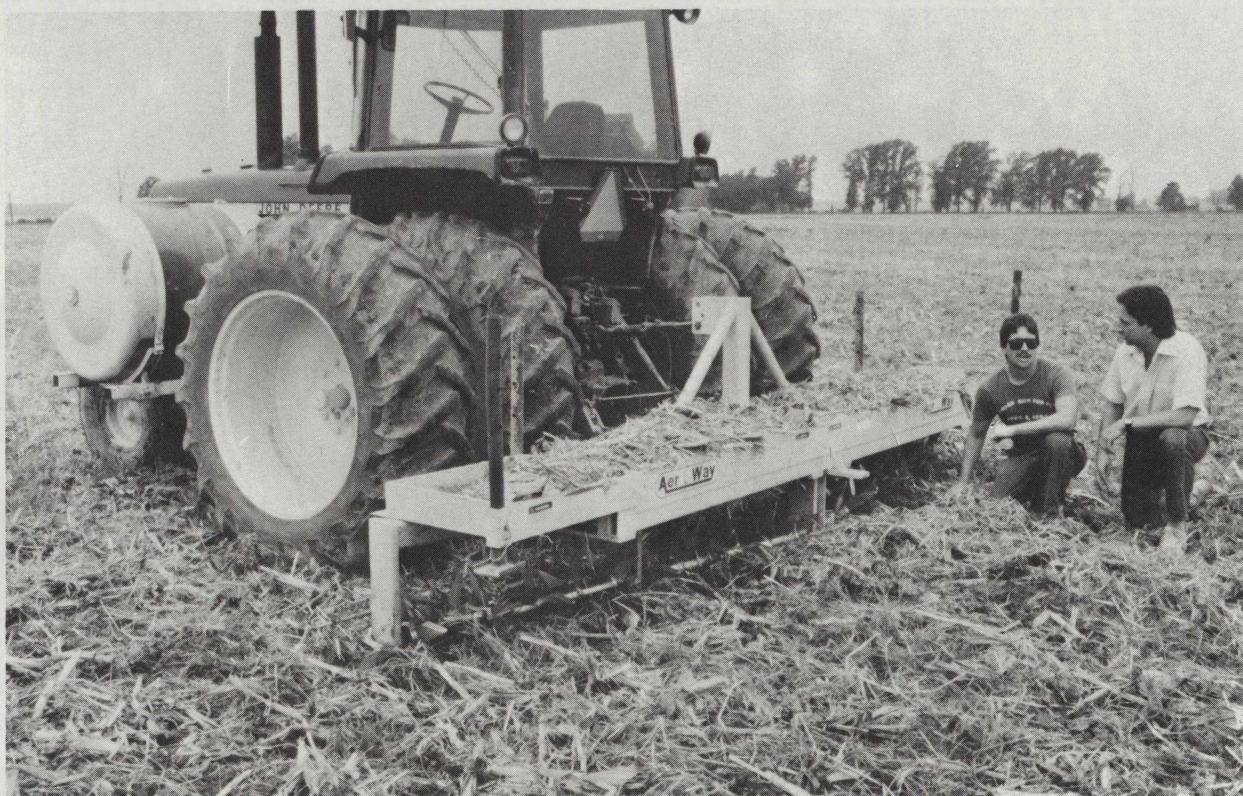
Strohm aerates the top 3 or 4 inches of soil with an Aer-Way, a single bar of rotating tines that can penetrate 7 inches deep.
