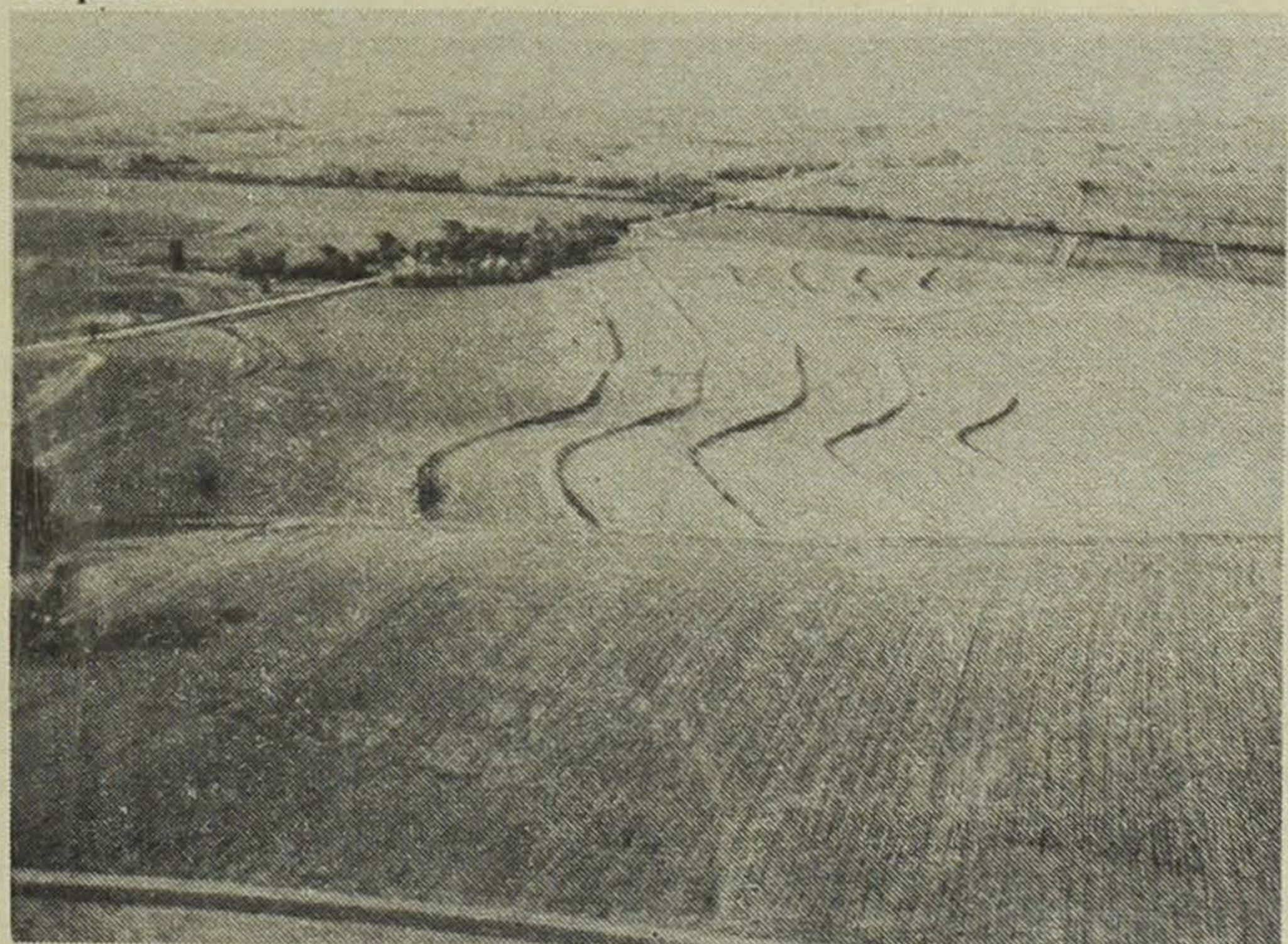
Tile outlet, parallel terraces protected this slope from erosion during the damaging storms of June 6, 14 and July 4 in Cass County.
