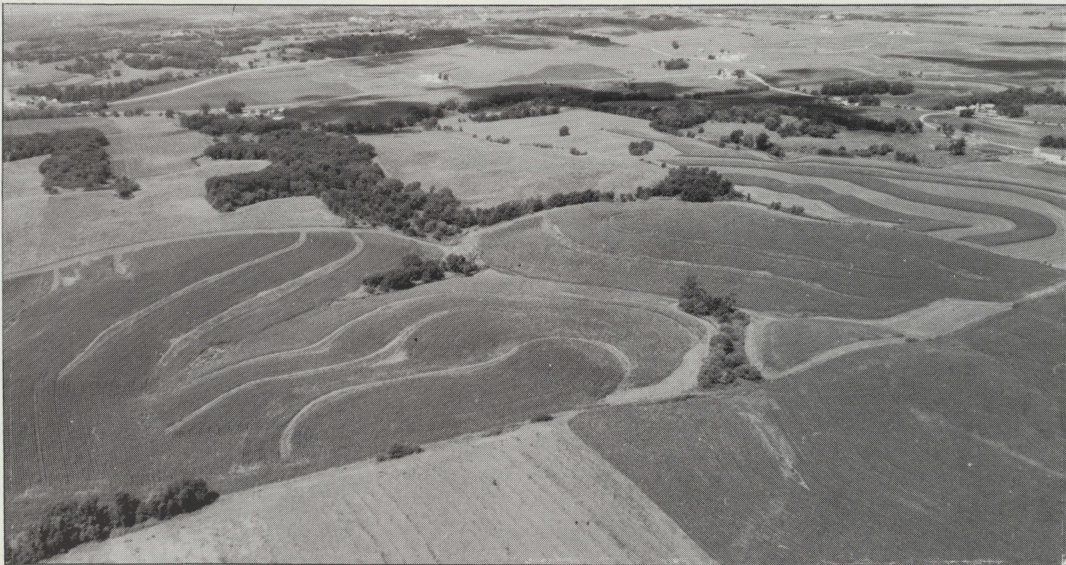
Joe Keith of rural Delhi installed narrow base terrace to control erosion, water runoff, and to maintain long term soil productivity.
