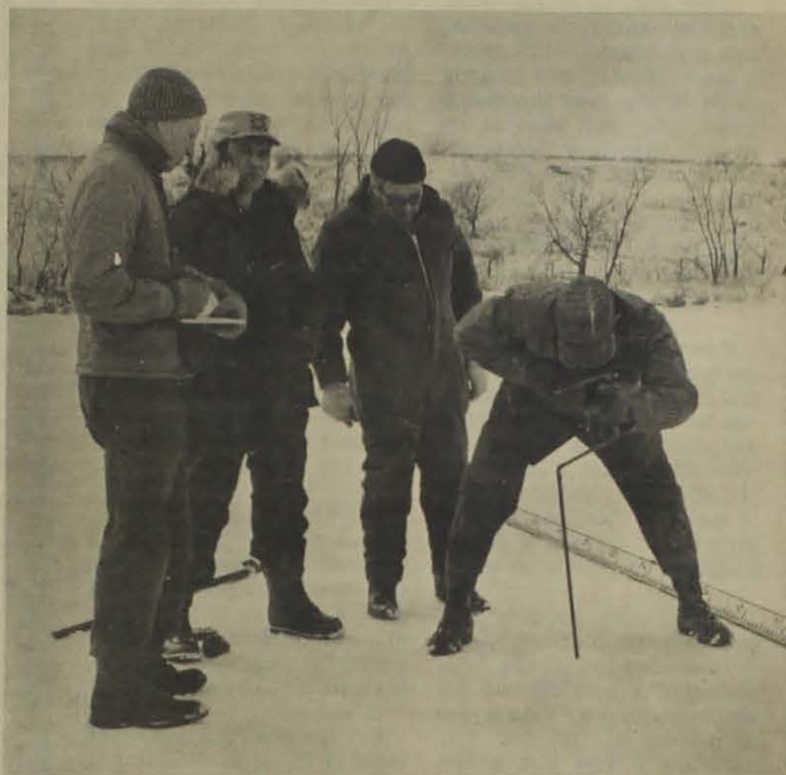
IT'S DEEP: A check is made of the depth of East Lake by members of a Soil Conservation Crew. T. J. Laing does the chore of cutting a hole through the ice as depth measurements are taken. The measuring rod is shown by his
