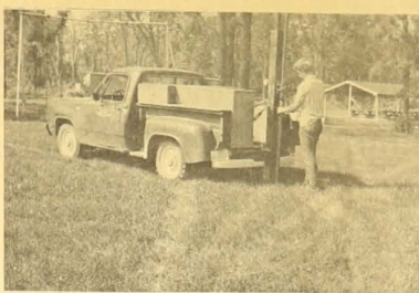
Probe truck used to provide additional information for soil survey and to test at depths up to 15 feet. Soil Scientist Walt Epler demonstrates use of the hydraulic powered probe which will be used in the Clayton County soil survey next year.
