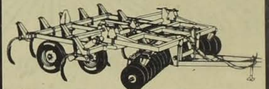
John Deere's Mulch Tiller has adjustable disk gangs for aggressive conservation tillage
