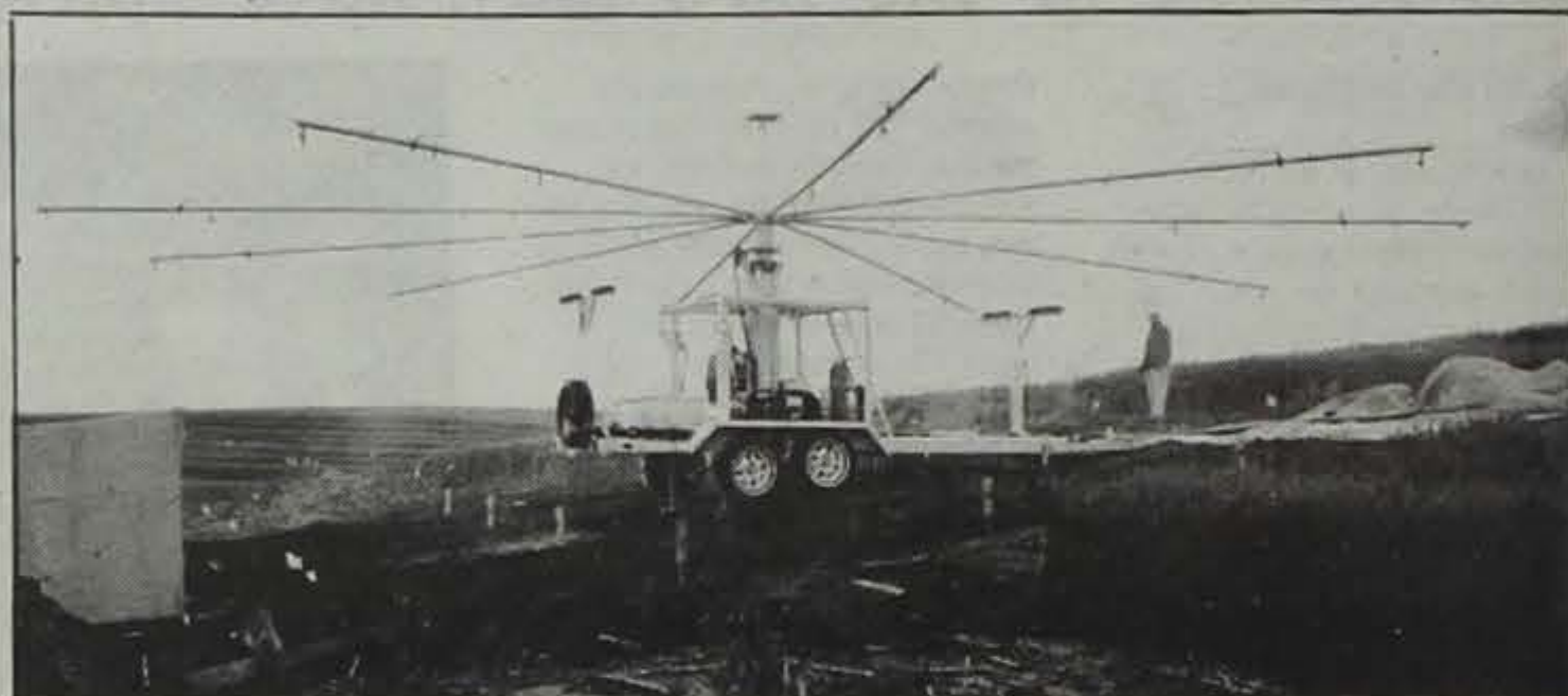
A "rain simulator", shown above, applies 2 1/2 inches of moisture per hour to prepared plots at the research farm. Runoff and soil-loss collection devices allow for water measurement and sampling. The results are then compared to field measurements of runoff from natural rainfall.
