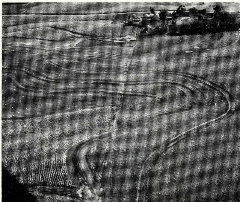
Terraces and farm pond on the Wayne Laughery farm in Seely township. A diversion above the pond carries farmplot drainage away from the pond. Note also where fence has been removed and terraces built through the old fence line. Field divisions are now on terrace lines.
