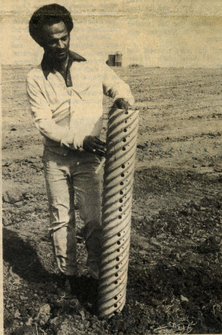
One of nine inlets on the Massner farm, this six foot metal pipe will drain two inches of runoff in 48 hours, or less, explained William Baugh.
