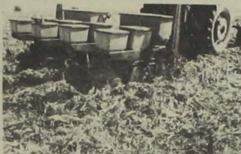
No-till means planting crops in last years crop residues without any primary tillage. Shown is a planter working in extremely heavy residues.
