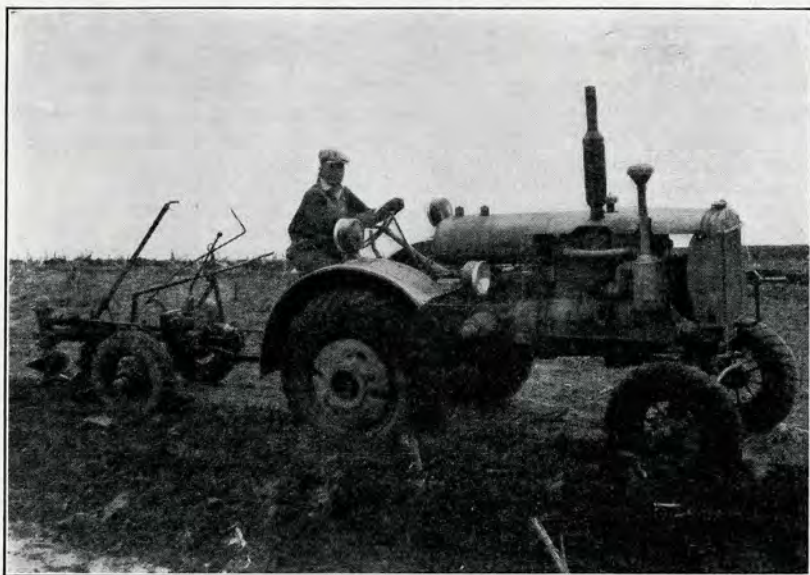
FIGURE 22.—The rotary-type terracer developed by the Agricultural Engineering Department of Iowa State College.
