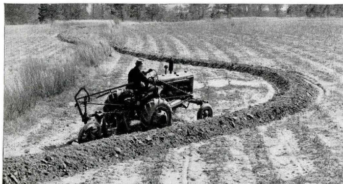
Starting and finishing a terrace with a disk plow.
