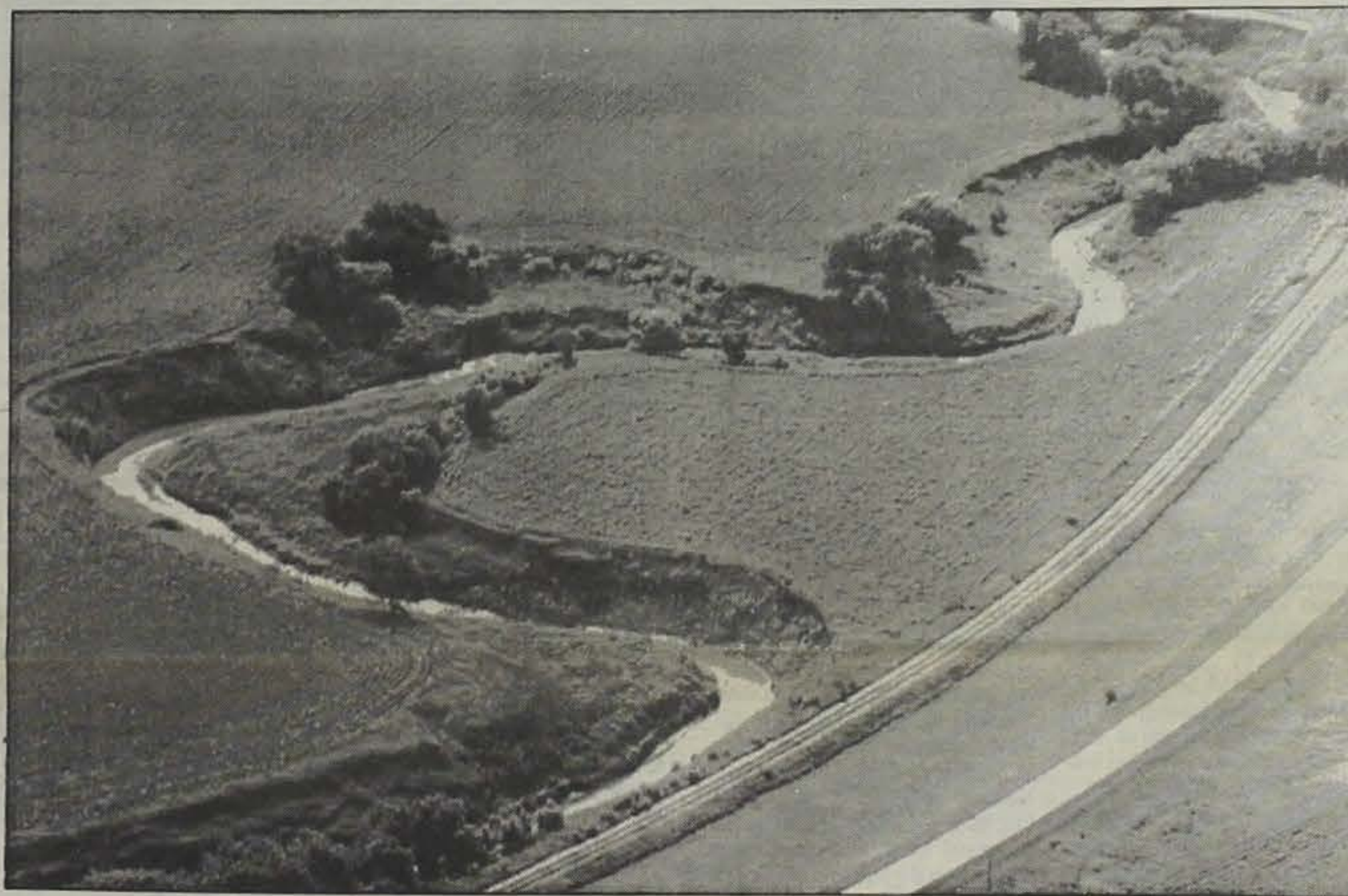
Mosquito Creek is each year coming closer to swallowing up this section of the only railroad line to serve the county. Repairs are expensive for all entities involved, and never ending, as well.
